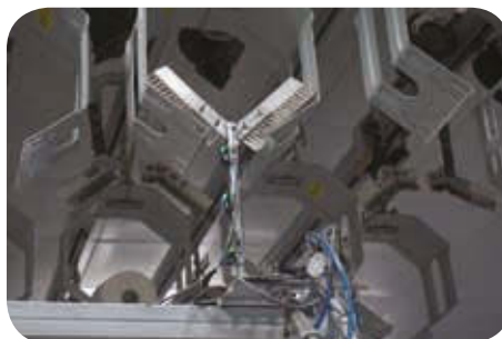
V-shaped brush designed and installed through technological improvement
