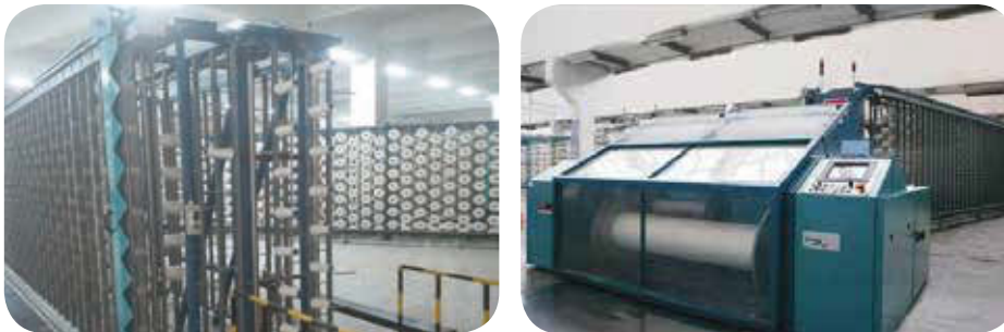
Benninger warping machine from Switzerland
